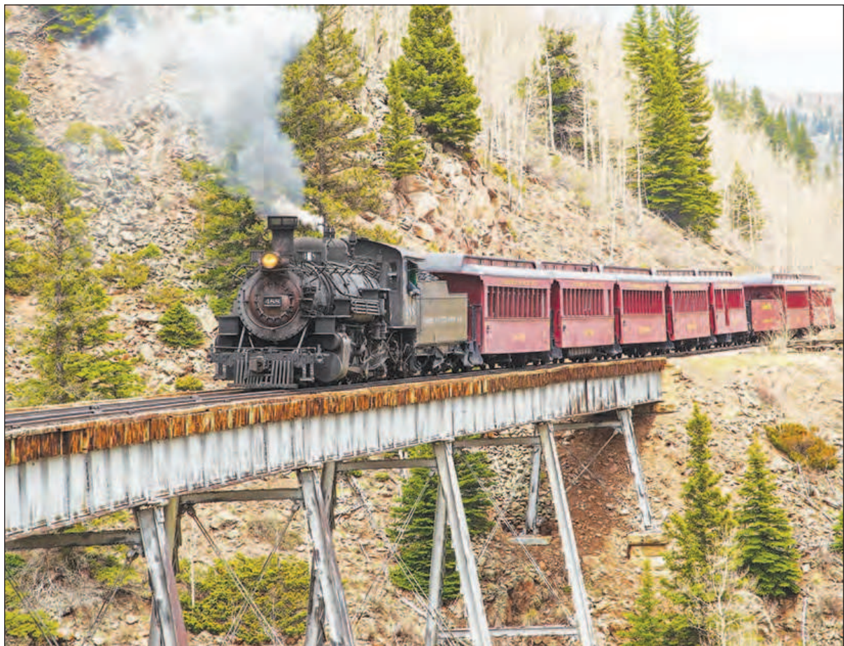
Cumbres and Toltec Scenic Railroad Engine 488 rumbles across the Cascade Trestle. At 137 feet high, it is the highest bridge on the 64-mile route between Antonito and Chama, N.M., and crosses Cascade Creek.
