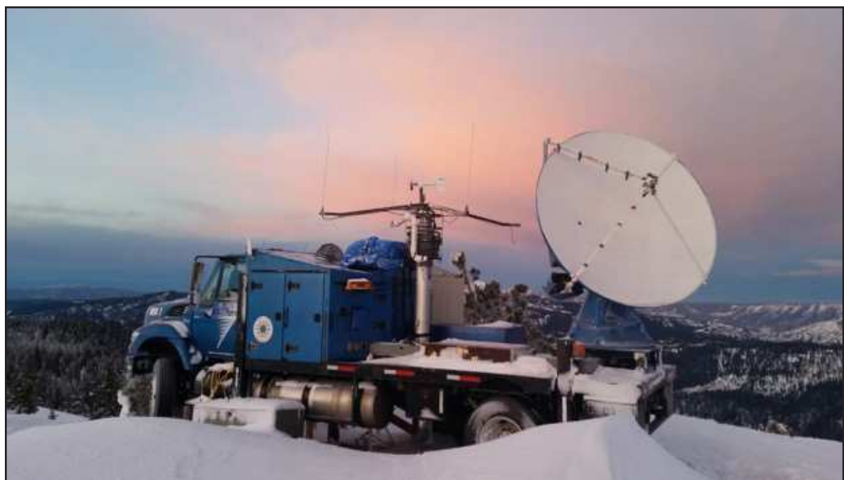
Courtesy photo by Joshua Aikins Researchers with the Seeded and Natural Orographic Wintertime Clouds: The Idaho Experiment (SNOWIE) project used a variety of tools to track cloud seeding events, including this "Doppler on Wheels" radar dish.
