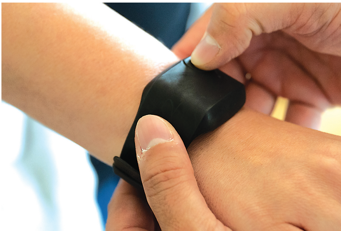
Student wearing E4 biosensor by Empatica that measures electrodermal activity, heart rate, movement and skin temperature.
