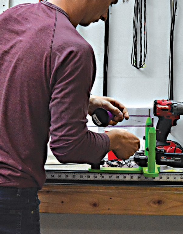
Adam Blakesley works on a custom bowstring in his work area in the back of the shop.
