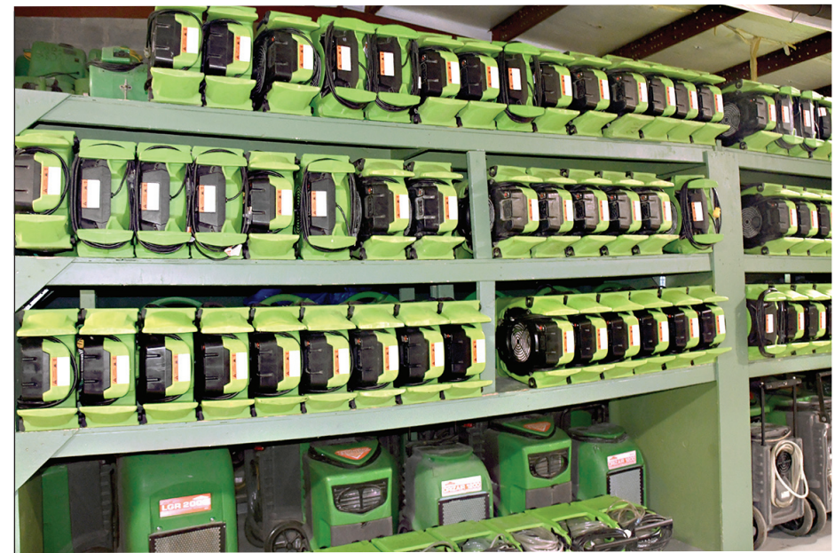
Having clean, well-organized equipment ready to go in a moment's notice is vital in the emergency clean-up business. Above, air movers and dehumidifiers sit ready to use.
