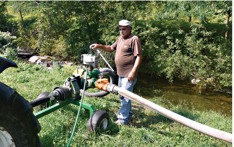
Bob Schmidt works the primer to get the pump working. The plants are automatically watered using a drip tape on raised beds.
