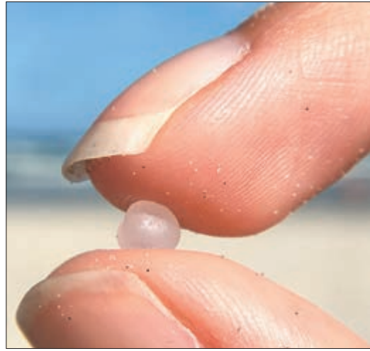
Small plastic particles called nurdles are shipped all over the world where they are melted down and molded into a variety of products and can pollute the oceans.
