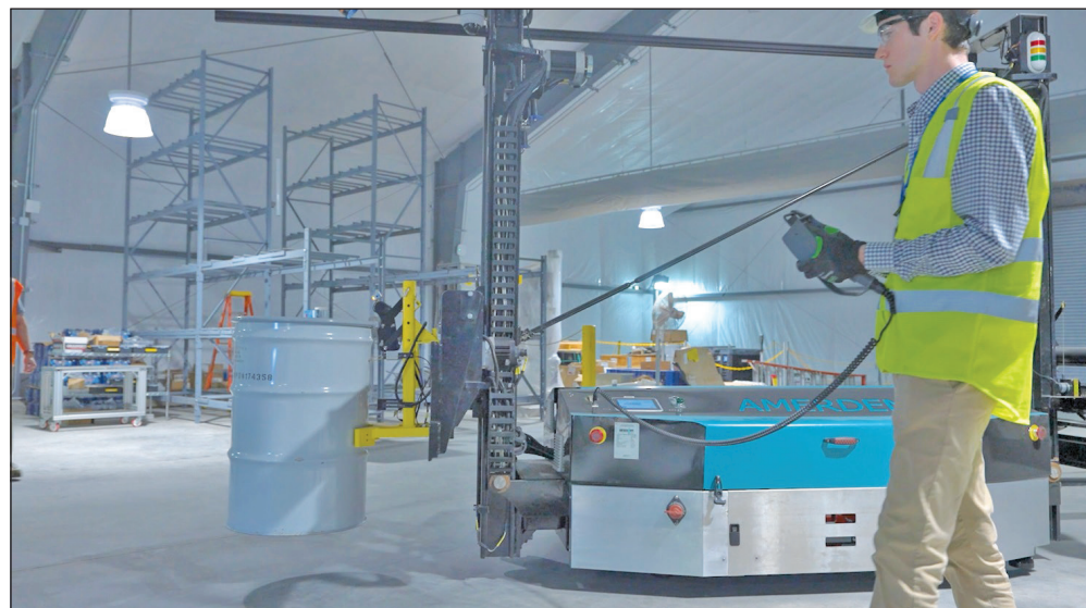
An Automated Guided Vehicle will be used to deliver shipping containers between staging and shipping inspection locations in a characterization and storage facility at SRS.
