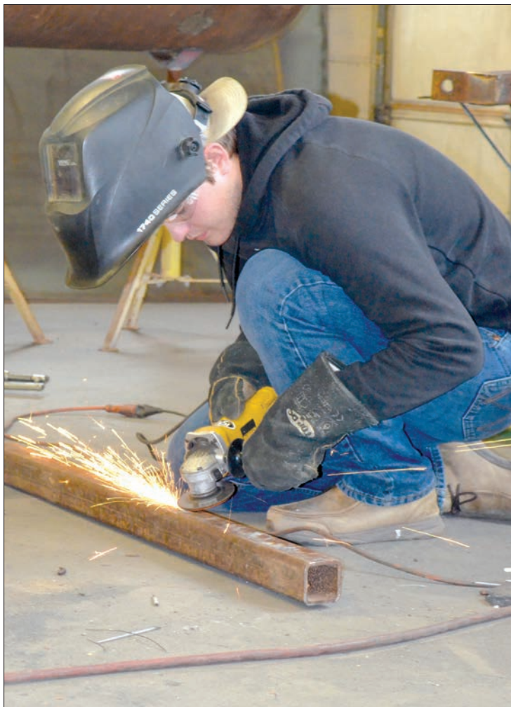
LISA PHELPS/PC RECORD-TIMES Caleb Hythe is using a grinder on some iron he is preparing to weld on a custom headache rack during an industrial tech/ag class.
