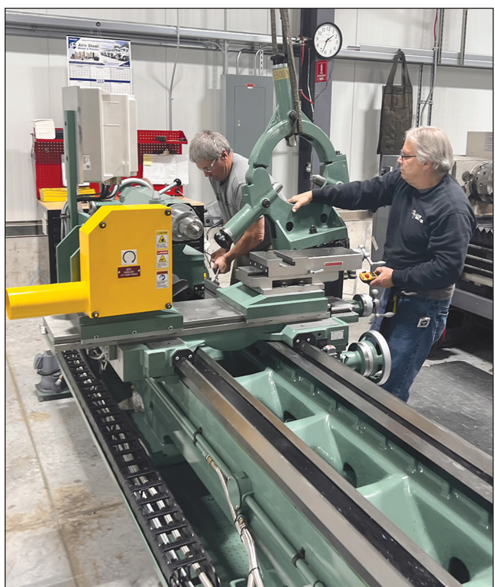
Veteran roll builders Craig Dinges, left, and Mike Fassig install the company's new Kingston Lathe. The custom lathe offers recipe storage and improves workflow by handling any sized roll or grinding specifications required by Black Bros. customers.
