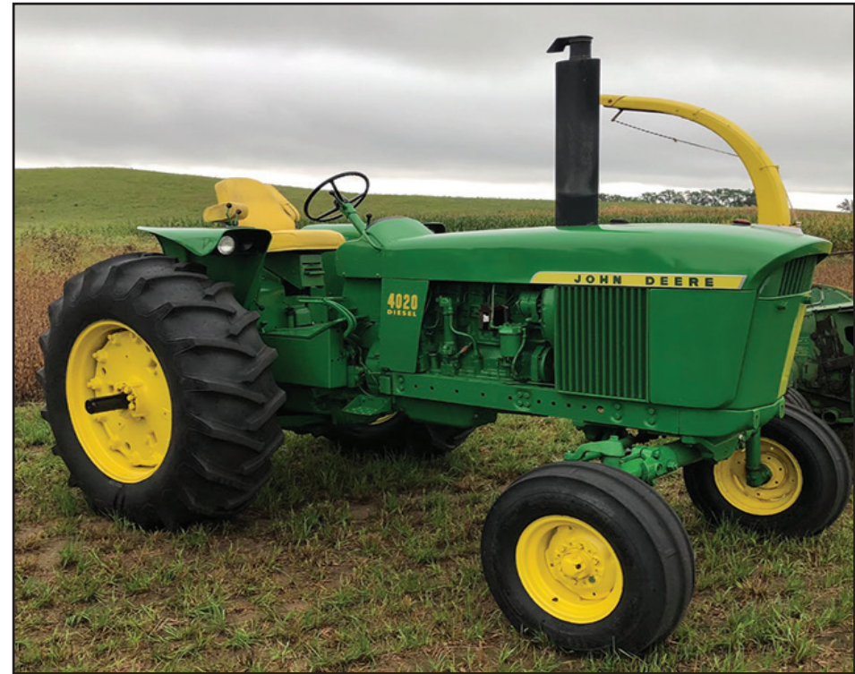
The John Deere 4020 was produced from 1964-1972. The tractor, which is nearly identical to its predecessor, the John Deere 4010, is offered three different engines, provided comfort in the cab, deluxe seats, and hydraulic controls to replace levers.
