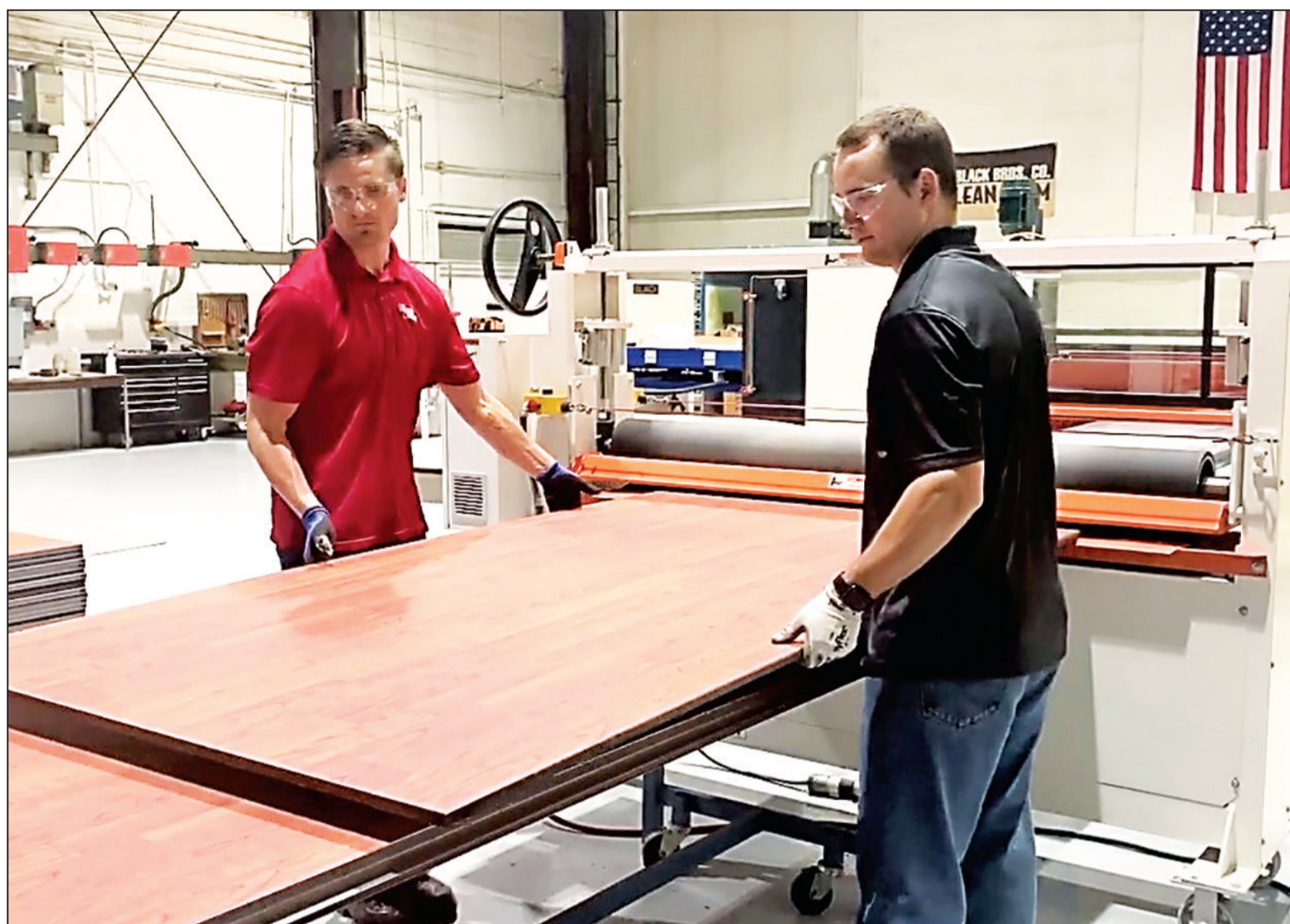
Black Bros. Co. System Representative Erik Weber, left, and Lab Manager Evan Carroll run a test panel through the Black Bros. Hot Melt Single Top Laminating System. The testing Lab is available to customers to run trials of Black Bros. machines with their materials.
