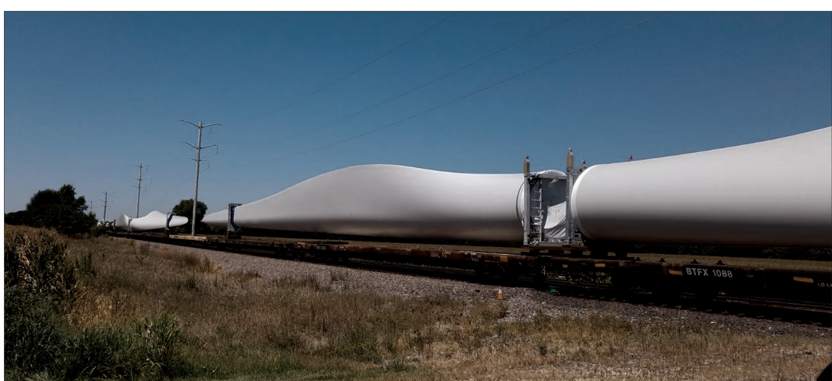
The only limit on size of wind turbines is the transportation mechanisms used. Here, wind turbines are being transported by rail through northern Illinois.
