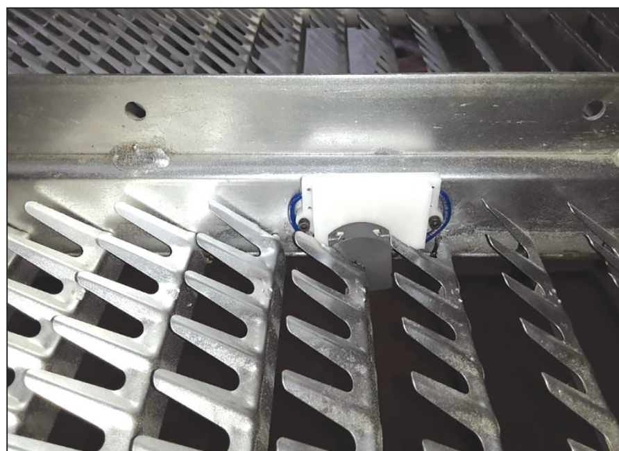
Utilizing closed-loop sensing technology, the SieveSense maximizes harvest efficiency through autonomous louver position adjustments on the fly.
