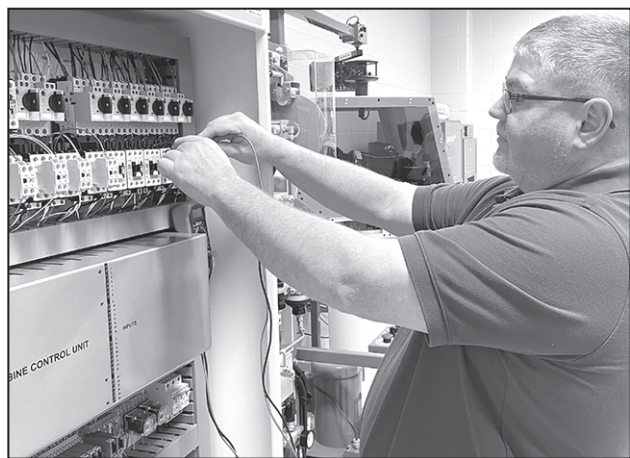
Wind technology instructor Steve Malavolti uses a multimeter to check a circuit on a Turbine Control Unit in IVCC's wind lab. (Photo contributed)
