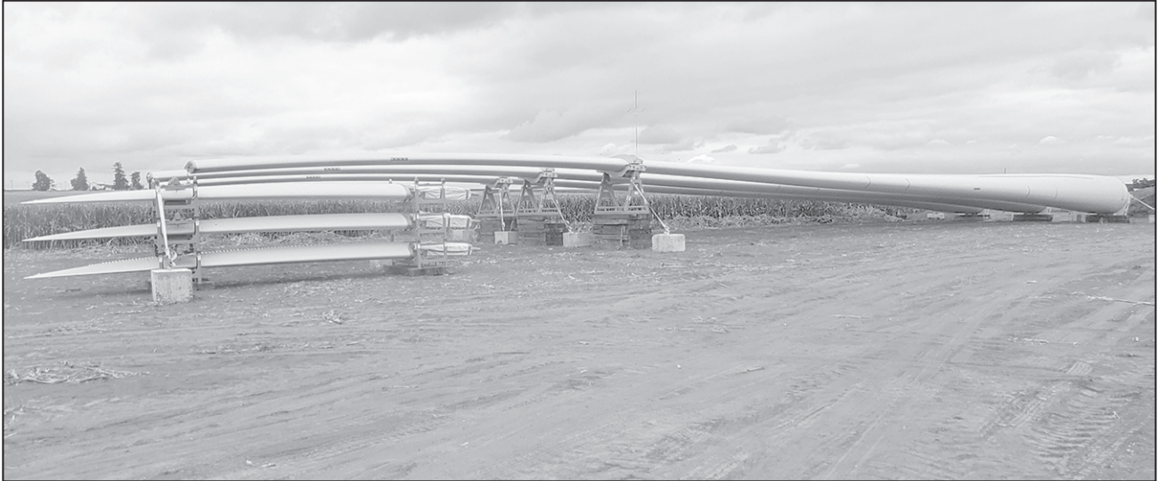
In the repowering process of wind turbines, 95 percent of the blades are being recycled. They’re made of fiberglass, wood, and other materials that can be recycled and reused. (Reporter photo by Brandon LaChance)
