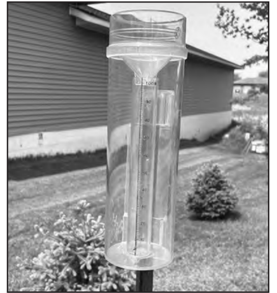
Precipitation observers are provided with a cylinder/test tube rain gauge, like this one located at the Rice SWCD office, in order to make sure all rain gauge measurements are the same.
