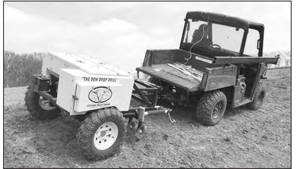
The Dew Drop Drill seeds bromegrass, timothy, and perennial rye grass on a water and sediment control basin in Rice County.
