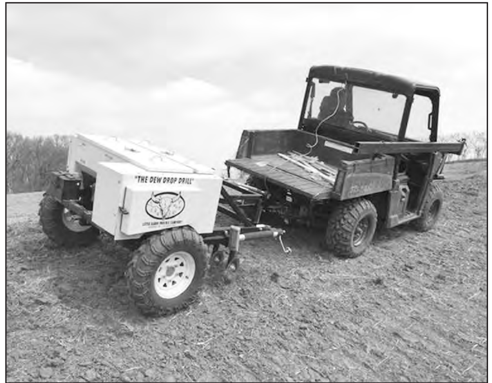
The Dew Drop Drill seeds brome grass, timothy, and perennial rye grass on a water and sediment control basin in Rice County.
