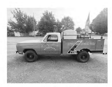
4 Wheel Drive 8 cylinder 360 CID, Automatic Transmission, Odometer states 16,487 but actual Miles unknown. Comes with a 200 gal tank, 23hp pump, and hose reel with 100' of booster line.
