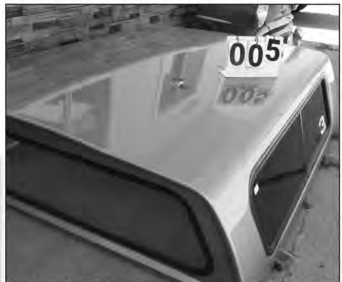
Glasstite Fiberglass topper, 21 1/2 high 68" x 96", light grey. Came off 2002 silverado ext cab, 2012 gmc sierra ext cab.
