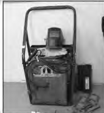
Lincoln welder, helmet, and welding vice - grips and gloves
